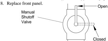
Figure 14 - Manual Shutoff Valve
